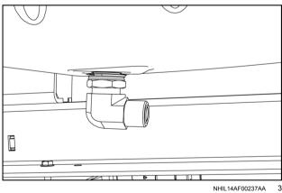
3. Remove the drain valve (1) from the bulkhead support bracket (2) by removing the lock nut (3).
