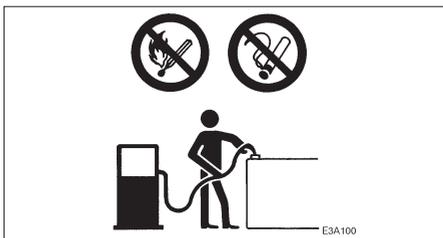
Keep flames away from fuel, hydraulic fluid, oil, grease and antifreeze. Fuel is particularly flammable and dangerous.
