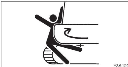
Never put your hands, feet or other parts of your body between the upperstructure and the undercarriage or tracks, between the machine body and working equipment, or between a cylinder and moving part. The size of these gaps change when the machine moves and if caught a person can suffer severe injury or death.
