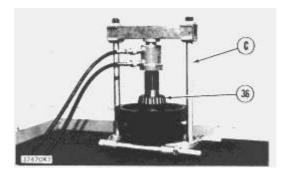
26. Using tool setup (C), remove the rear bearing cone (36) and idler gears from shaft.
