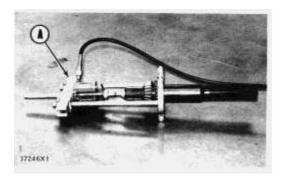
7. Remove bearing cup (10) from shaft. Using tool setup (A), remove the bearing cones from the output shaft.
