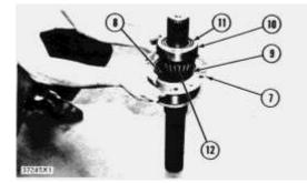
5. Remove the cage (7) and output shaft from the housing.
