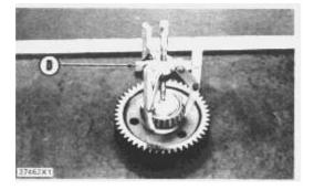
**29.** Using tool setup (D), remove the two bearing cones from output gear (34).
