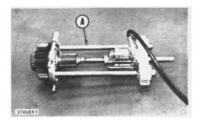
**36.** Using tool setup (A), remove the two bearing cones from input gear (41).
