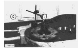
d) Install the cage retaining bolts and locks. Tighten bolts to  $65 \pm 5$  lb. ft. (9,0  $\pm$  0,7 mkg). Using indicator group (C), check the end play of input gear.
