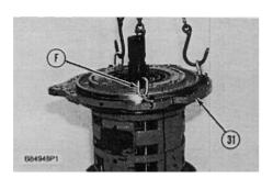
**24.** Fasten tool (F) and a hoist to manifold assembly (31) as shown. Remove manifold assembly (31) from the No. 3 and 4 clutch housing. The weight of the manifold assembly is **88 kg (194 lb).**
