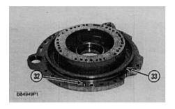
25. Remove dowel (32) and O-ring seal (33) from the manifold assembly.
