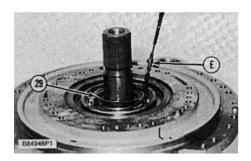
**NOTE:** After retaining ring (29) has been removed, the housing assembly will drop a small amount into the manifold assembly.
