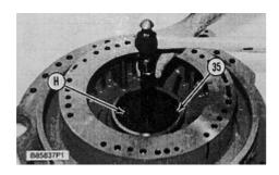
27. Use tool (H) to remove bearing (35) from the manifold assembly.
