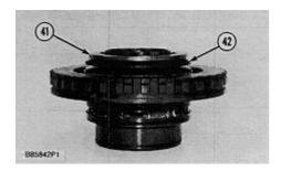
33. Remove retainer plate (41), and three disc springs (42) from the housing assembly.
