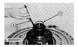
18. Use tool (D), and remove retaining ring (17) from the output shaft assembly.
