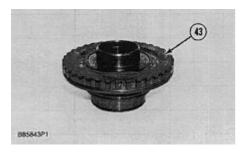
**34.** Remove clutch piston (43) from the housing assembly.
