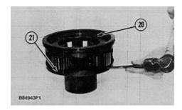
**b.** Use a hammer and a punch to push spring pin (21) into planetary shaft (20).
