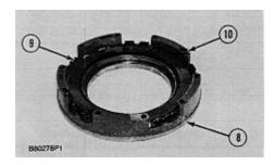
13. Remove reaction dowels (10) and clutch piston (9) from No. 6 clutch housing (8).
