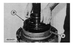
**30.** Remove housing assembly (39) from ring gear (38).
