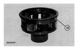
**a.** Remove seal ring (19) from the carrier.
