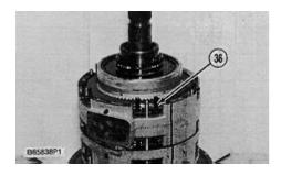
**28.** Remove springs (36) from the clutch piston.
