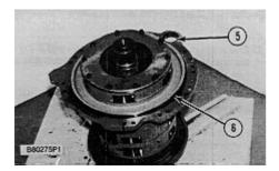
**8.** Remove two O-ring seals (5) and O-ring seal (6) from the manifold assembly.
