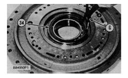
**26.** Use tool (G), and remove retaining ring (34) from the manifold assembly.
