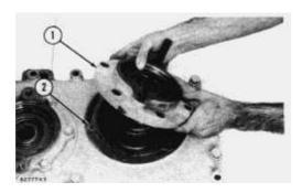
**1.** Remove the six bolts that hold bearing cage (1) to the cover. Install two 5/8"-11NC forcing screws and remove the bearing cage and shims (2).
